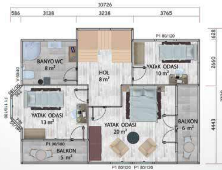
77m 2 (66m 2 + 11m 2 BALKON) 1. KAT PLANI 77m 2 (66m 2 + 11m 2 Balcony) First Floor Plan
